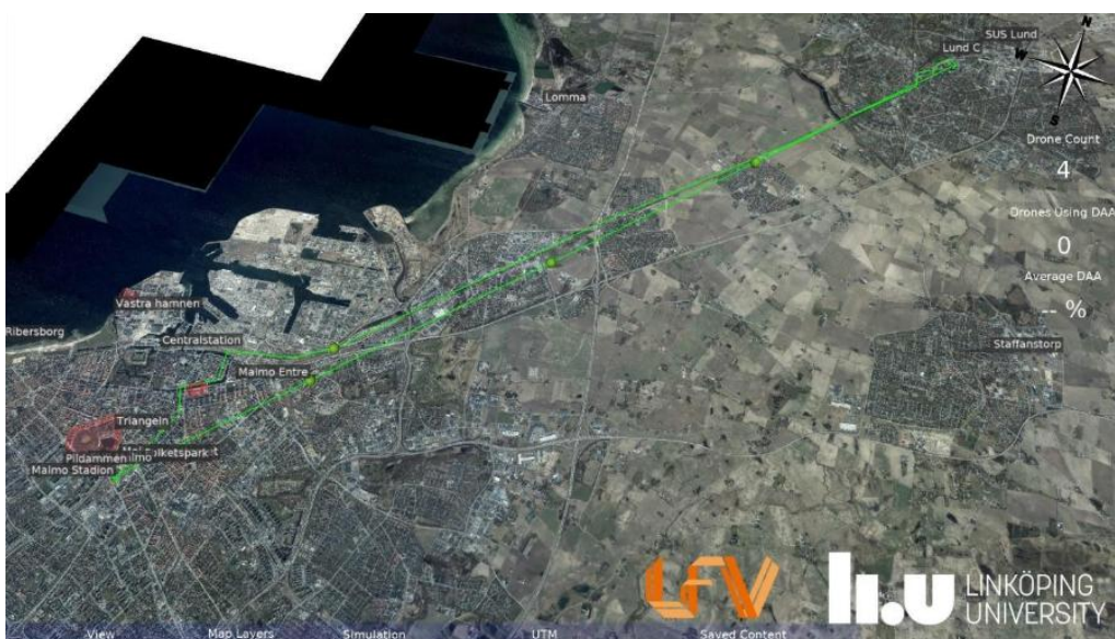
Figure 7 overview of use case “extended rorpost” two route options between Malmö hospital and Lund hospital. Straight line vs routing via waterways out of Malmö, over the central station and along the railway tracks to Lund
