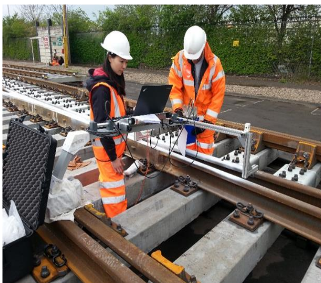
FIGURE 12. SWITCH SET OF POINTS MEASURED AT BEESTON WITH PAINTED SURFACE (UPPER-LEFT); DETAILS OF A MARKER PLACED ON PAINTED CROSSING WING SURFACE (UPPER-RIGHT); TROLLEY MEASUREMENT AND OPERATION ON CROSSING PANEL ASSEMBLY (BOTTOM-LEFT); ILLUSTRATION OF PLACEMENT OF MARKERS ON CROSSING (BOTTOM-RIGHT)
