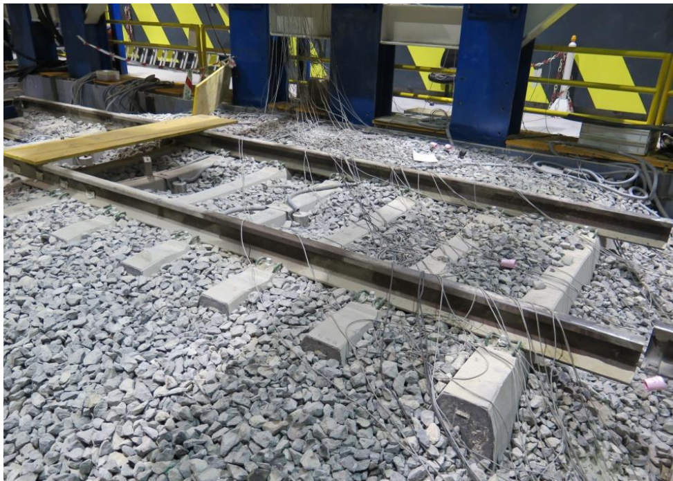
FIGURE 20. BALLASTED TRACK PREPARED FOR THE VHST TESTS
