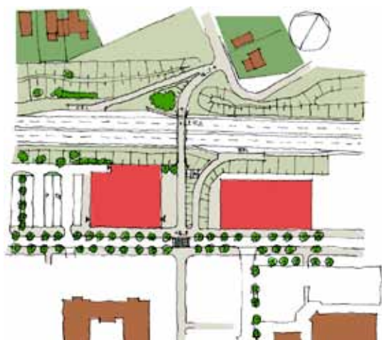
Illustration of the alternative plan for Riksväg 55 at lowered elevation. From Uppsala Workshop – Highway 55, Kvarnbolund–Berthåga section.
