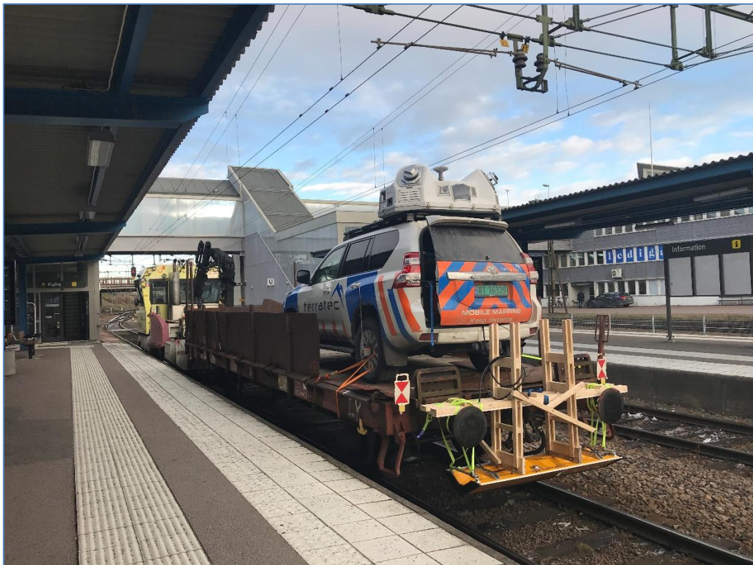
Figure 2 3DR - DXG Georadar attached to Railway cart
