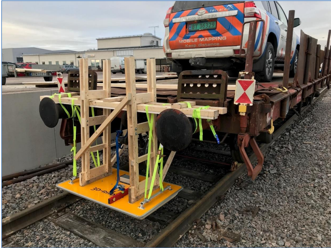
Figure 1 3DR - DX Georadar attached to Railway cart
