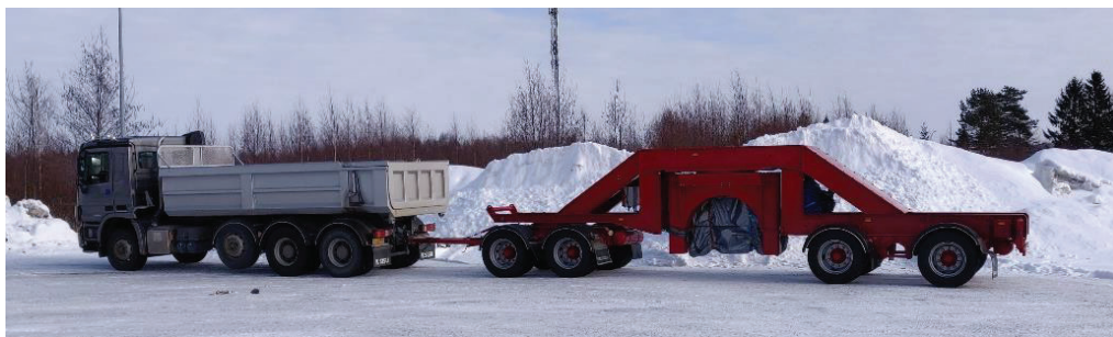
Figure 2. Tire testing trailer of University of Oulu
