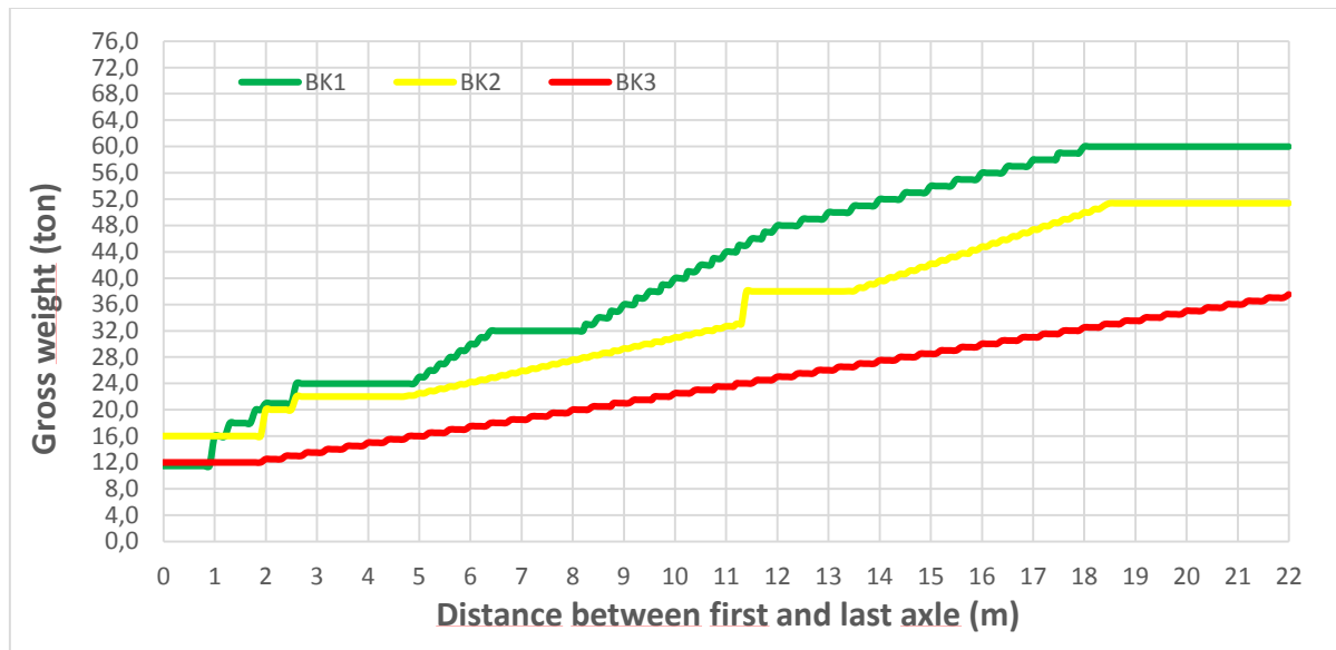
Figure 2. Permissible gross weight vs. distance between first and last axle of the vehicle, for the three bearing capacities (Trafikverket 2014)
